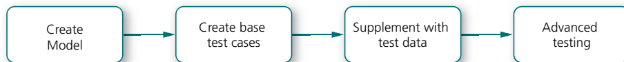
Figure 8.1: Process for test design in four steps. We start with an analysis of the test basis and creation of a model. Then we cover the model, supplement it with test data, and end with the advanced testing which is perhaps not always covered by the model.
